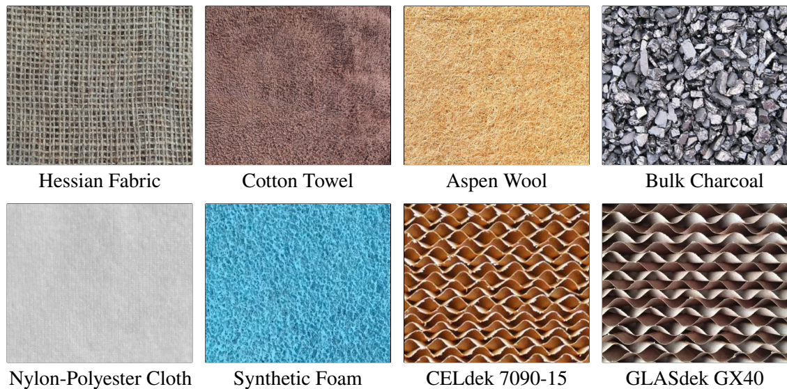
Figure 2.17: Selected samples of common materials used for convectional pads [58, 59, 60, 61].
