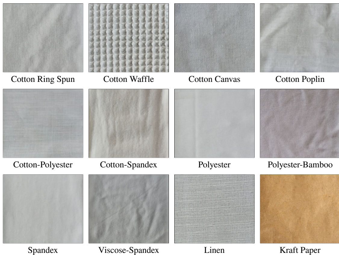
Figure 5.38: Samples of the selected materials used for deciding the fabric of the cooling pad. (The hessian (similar to jute) was included previously in Figure 2.17 with examples of conventional pads).
